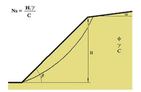
This parameter is a key factor for estimating the angle of slope stability. Ns is interpolated from the results of a series of limit equilibrium slope stability analyses carried out by Fang et al. (see below).
