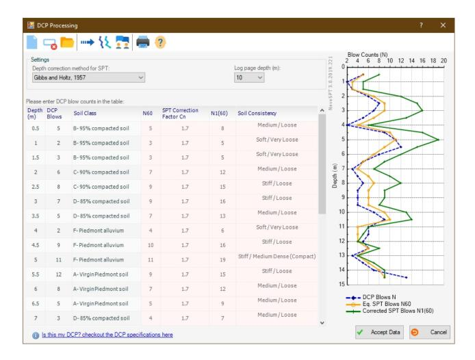
The following chart presents the correlations between DCP blows per increment and standard SPT blow counts for different soil types.
