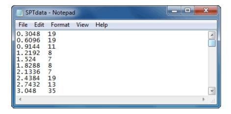
where, 0.3048, 0.6096, 0.9144, etc are depths and 19,19,11, etc are corresponding blow counts per foot (N). Text files can be easily generated using Windows **Notepad** or by exporting your data from spreadsheet applications such as Microsoft Excel into text format. For soil layers text file, each line consists of layer *thickness*, its *unit weight*, *soil type*, *D50* and *OCR* separated by comma.
