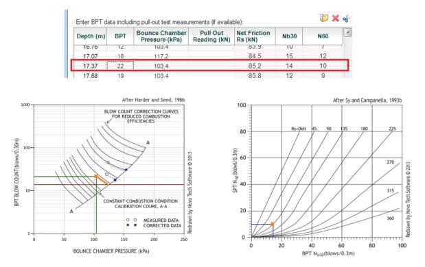
At a depth of 17.37 m, BPT=22 and bounce chamber pressure P = 103.4 kPa. This point (BPT,P) is shown on the left chart by an orange square and two green lines. An orange line parallel to the closest contour shows the intersection with line A-A. The horizontal red line is drawn from this point to find the corrected BPT on vertical axis.
