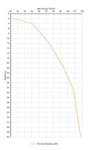
'Net Friction' = 'Measured Friction - ('Weight of Bit' + 'Weight of Scale Coupler' + 'Weight of Casing Per Unit Length' \* Z)
